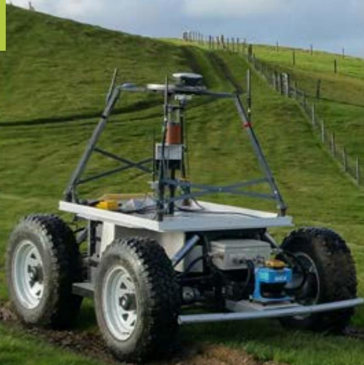
Idris is a four wheel drive and steering electric vehicle. The main use of Idris is for the Department of Computer Science's research in field robotics and in particular visual navigation.
